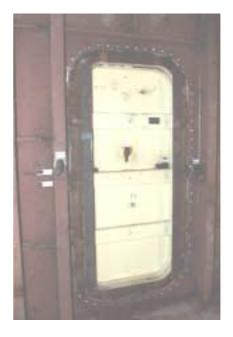
Figure 13 A level I door in its test frame
