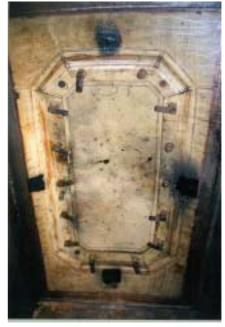
Figure 23 The Prima Membrane Mk3 door in the DERA Blast Test box (Post Trial).
