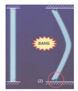
Figure 10 High Stress and Strain at the BHD & Deck connection
