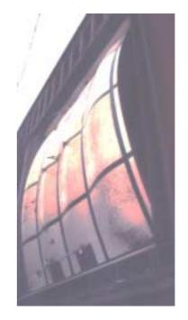
Figure 28 The large deflection of the conventional bulkhead equipped with curvature limiters, tested at Meppen (Germany) without cracks.
